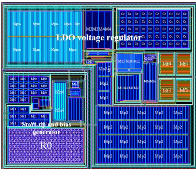
Figure 15. Integrated LDO Chip Layout
